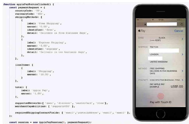
Tampering with a transaction amount via a Man-in-the-Middle attack
