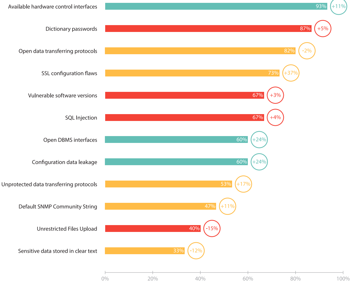
Ten most common vulnerabilities at the network perimeter
